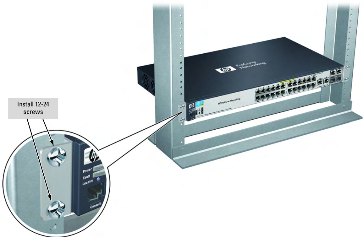
Figure 2-4. Mounting in a rack
