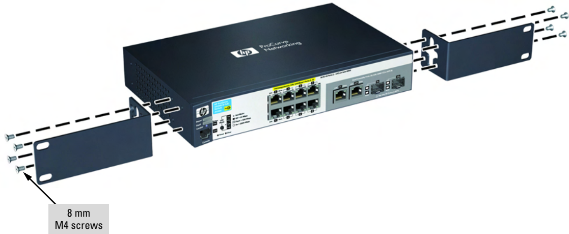
Figure 2-5. Attaching mounting brackets
