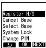
6. Press **NEXT** to display the second screen, select "Enable CS Web", and then press **OK**.
