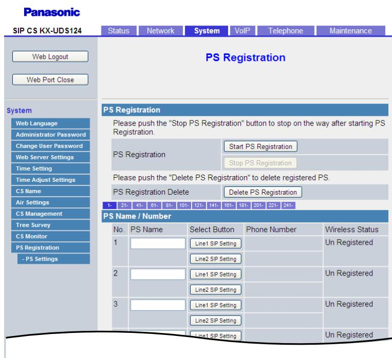
1. Log in to the Web user interface for the Super Master CS (→ see **2.1 Web User Interface Programming**).
